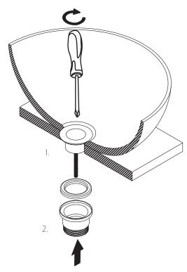
Connect pipe work and refit the lid and grate onto the waste.
